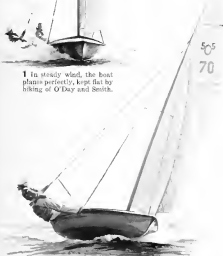
2 In rising wind, O'Day drives (veers) off and stacks main. Both hike out farther.
